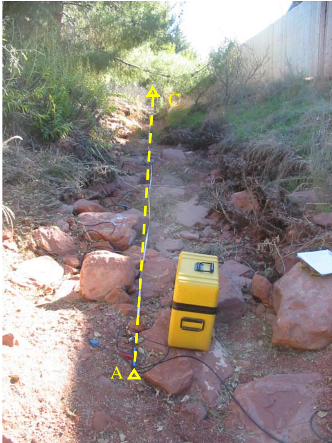
Figure 10; Photo 1: Seismic Survey Line HW3-S04 view looking toward the North along existing drainage channel from geophone A toward geophone C.
