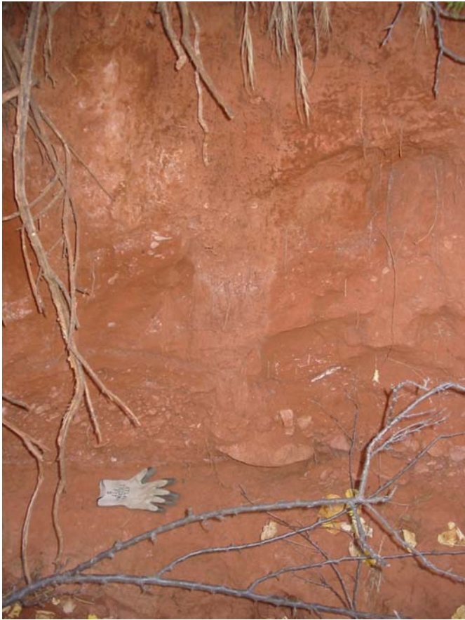
Figure 11a; Photo 1: Silty-sand with gravel alluvium derived from the weathering of the Supai Formation in the vicinity of HS3-S02.
