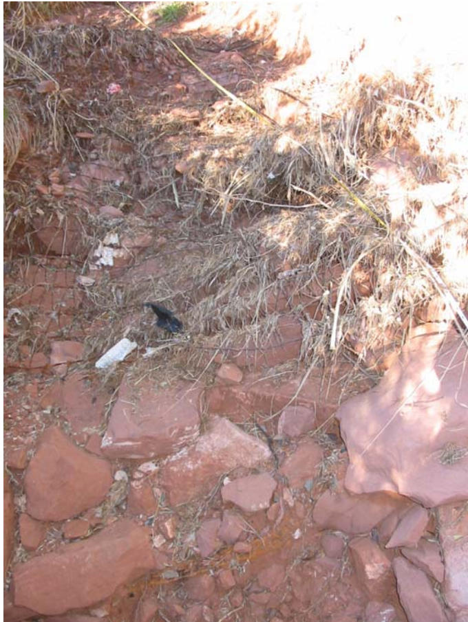
Figure 11b; Photo 1: Failed erosion protection located in the vicinity of seismic survey line HW3-S04.
