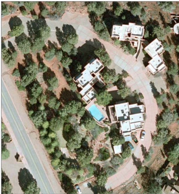
Example of a 12 unit development on less than two acres. The four buildings are clustered together leaving an open space buffer along the road.
