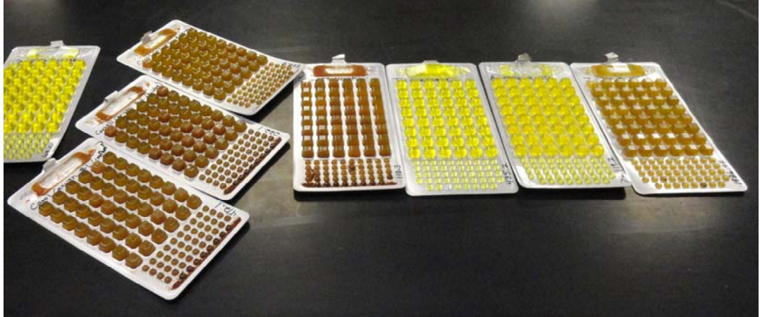
Figure 12. Quanti-trays showing variation in sediment yield among stormwater flow collected from Sedona’s washes on August 1. The darker brown the sample is, the more sediment it holds. From left (downstream) to right (upstream) are Carroll Canyon 1, 2, and 3, Soldier’s Wash, Tlequepaque, Arroyo Roble and Jordan Wash. (The sample on the far left is from Cornville Bridge, where the storm pulse had not reached yet.)
