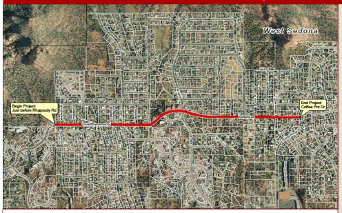
The project will include a mill and overlay, with minor shoulder widening and curb along the south side of the roadway allowing for the construction of a shared use path in the future. The approximate one mile segment of Sanborn Drive/Thunder Mountain Road is between Rhapsody Road and Coffee Pot Drive.
