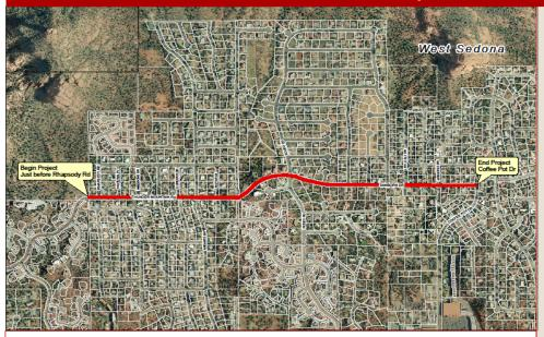
The project will include a mill and overlay, with minor shoulder widening and curb along the south side of the roadway allowing for the construction of a shared use path in the future. The approximate one mile segment of Sanborn Drive/Thunder Mountain Road is between Rhapsody Road and Coffee Pot Drive.
