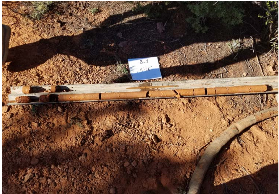
Photograph 1: Sample cores B-1, 11 through 16 feet.
