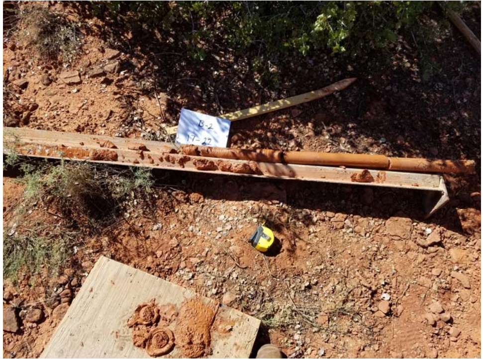
Photograph 5: Sample cores B-2, 17 through 22 feet.
