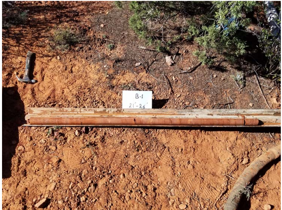
Photograph 3: Sample cores B-1, 21 through 26 feet.
