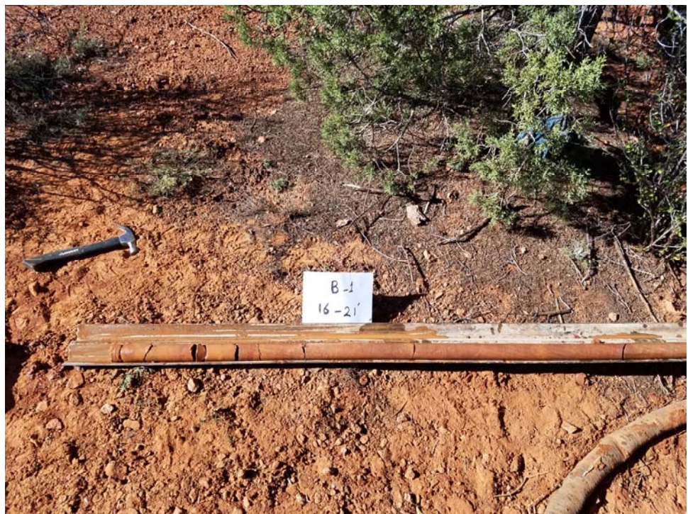
Photograph 2: Sample cores B-1, 16 through 21 feet.
