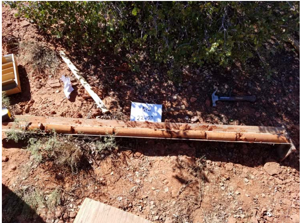
Photograph 6: Sample cores B-2, 22 through 27 feet.
