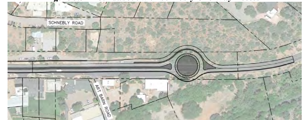
Figure 3.4 - Roundabout No Schnebly One Way Access
