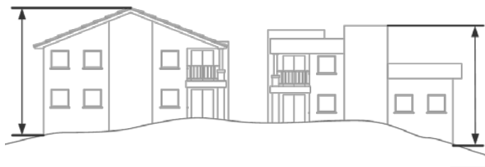
Figure 2-7: Maximum Overall Building Height
