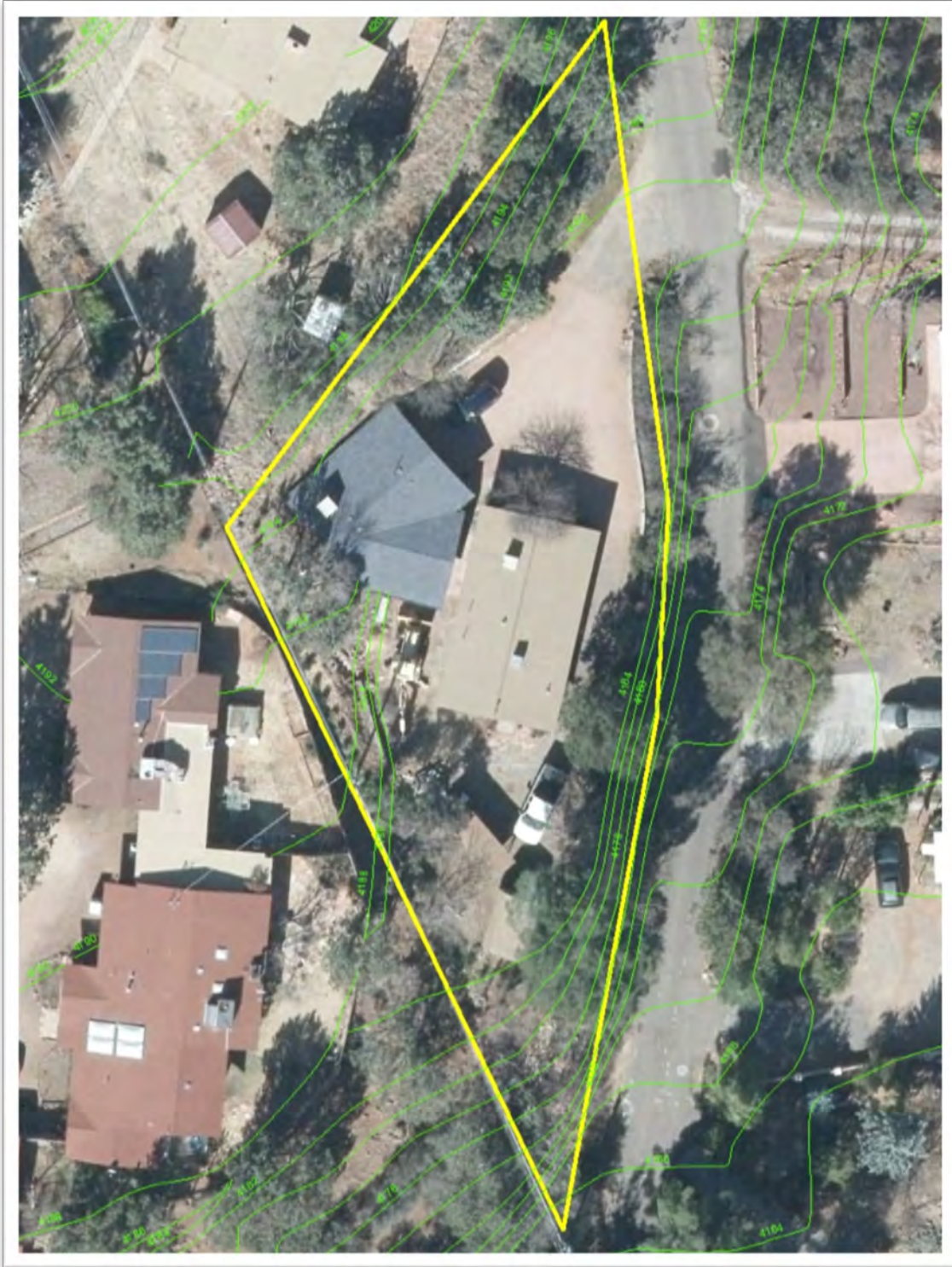
Figure 5: Contour map of property, showing grade difference between street and surrounding properties.
