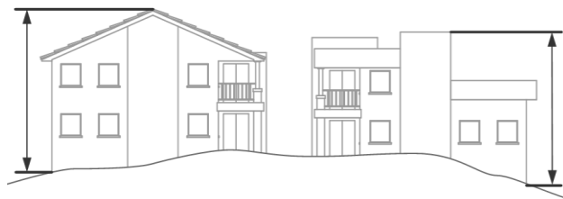
Figure 2-7: Maximum Overall Building Height
