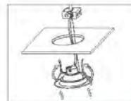
Push clips up & install into opening
