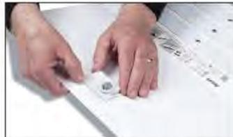
Step 5: Insert the sensor back into the hole. The sensor may or may not require a socket.
