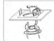
Push clips up & install into fixture
