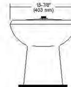
**NOTE:** All vitreous china dimensions shown in these drawings are nominal. Dimensions can vary within the tolerances established in the governing ASME A112.19.2/CSA B45.1 standard. Please take this into consideration when planning rough-in and plumbing layouts.
