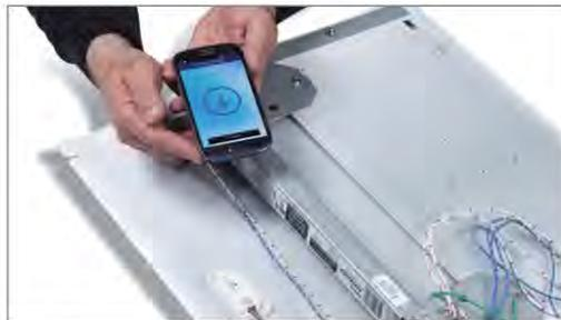
Step 1: Place the smartphone next to the NFC antenna on the driver.
