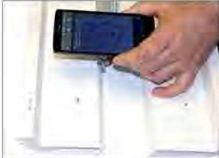
Step 1: Place the smartphone next to the NFC antenna on the driver.
