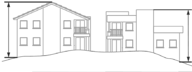
Figure 2-7: Maximum Overall Building Height
