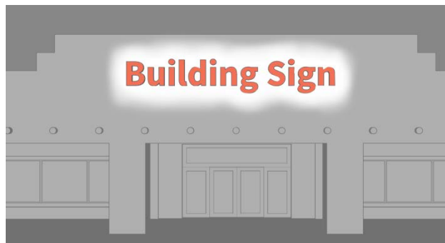
Figure 6-9: Individual Halo-Lit Letters with Opaque Face
