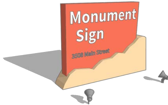
Figure 6-8: Ground Mounted Uplighting of Monument Sign
