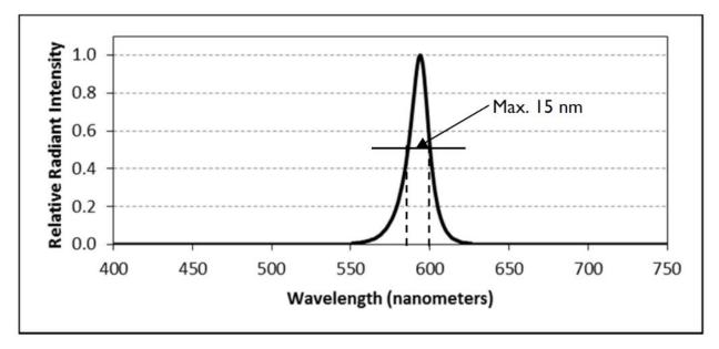
Phosphor-Converted Amber LED (PCA LED)
