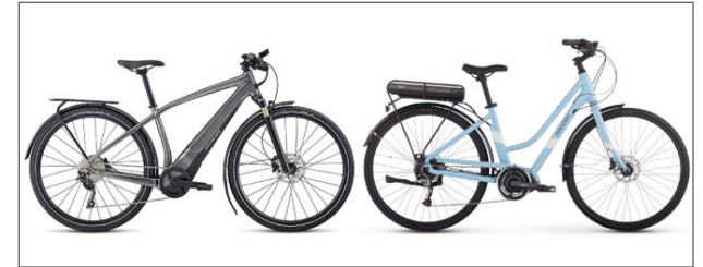
E-bikes have a battery and motor that can be integrated into the bike frame.
