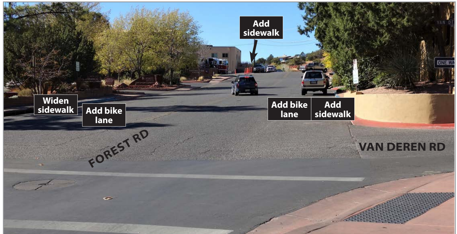
Figure 1. Forest Rd potential "Complete Street" improvements
