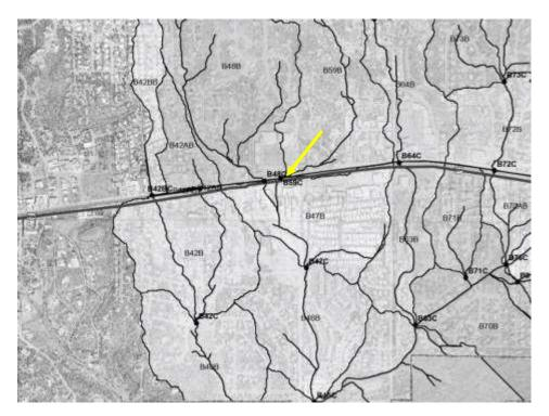
The model was constructed using 1 sq. ft. areas using an AutoCAD surface built from the City of Sedona Topography resulting in an accurate representation of post-development conditions. Below is a visual image of the model built to represent the 100-yr flood.
