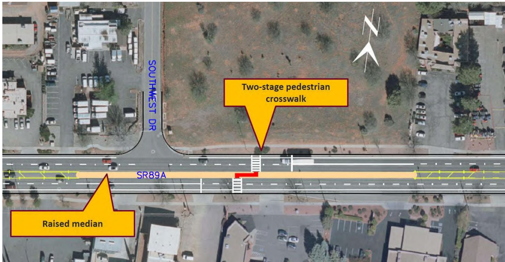
Figure 4.16: Example of a Two-Stage Pedestrian Cross-walk
