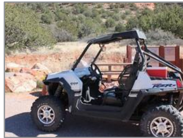
UTV (Utility Task Vehicle), ROV (Recreational Off-highway vehicle), or “side-by-side”, such as Polaris RZR®. Features steering wheel and roll-bar.
