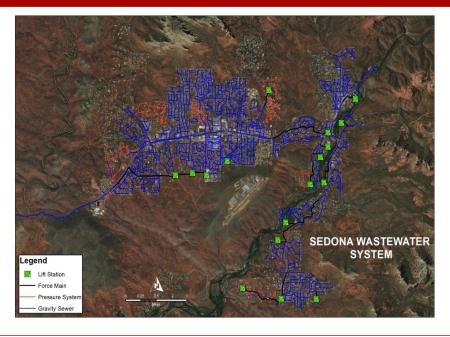
The 2017 Wastewater Master Plan Update (WWMP) included condition assessments of existing sewer infrastructure. During the evaluations, several areas were identified as needing attention. This project will rehab or replace sewer line scattered throughout the city. Design is scheduled for FY21-22, while construction is scheduled for FY22-23.
