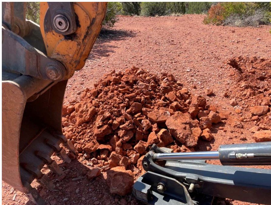
Photo 4 – View of material excavated from Test Pit 2 over the depth range of 0.0 to 1.5 feet, which appears to be primarily excavated mudstone bedrock.
