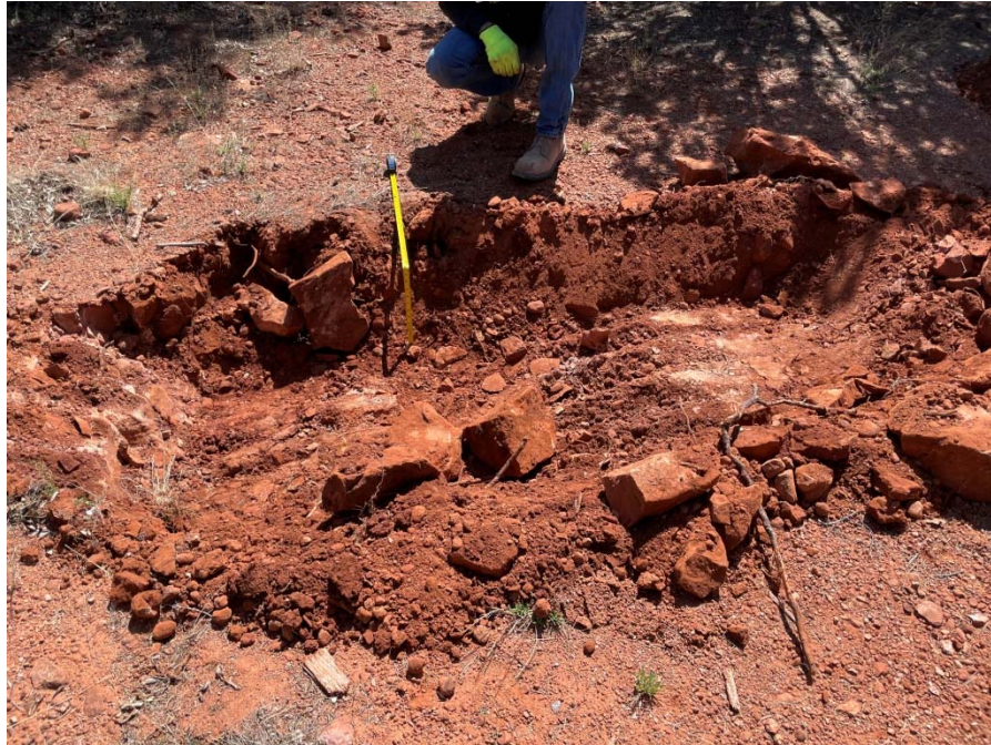
Photo 11 – Excavated Test Pit 6. Test Pit 6 was terminated at a depth of 1.0 feet due to backhoe refusal on hard mudstone bedrock – Supai Formation. . The upper 1.0 feet of red clayey gravel with sand and cobbles is medium dense, damp, PI of 10.
