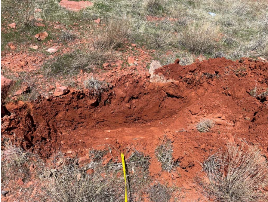
Photo 13 – Excavated Test Pit 7. Test Pit 7 was terminated at a depth of 1.0 feet due to backhoe refusal on hard mudstone bedrock – Supai Formation. . The upper 1.0 feet of red clayey silty sandy gravel with cobbles is medium dense, damp, PI of 4.
