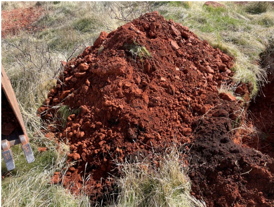
Photo 18 – View of material excavated from Test Pit 9 over the depth range of 0.0 to 2.5 feet.
