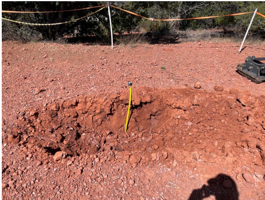
Photo 3 – Excavated Test Pit 2. Test Pit 2 was terminated at a depth of 1.5 feet due to backhoe refusal on hard mudstone bedrock – Supai Formation. . The upper 1.5 feet of red clayey silty gravel with cobbles, some sand is dense, probable highly weathered mudstone bedrock.
