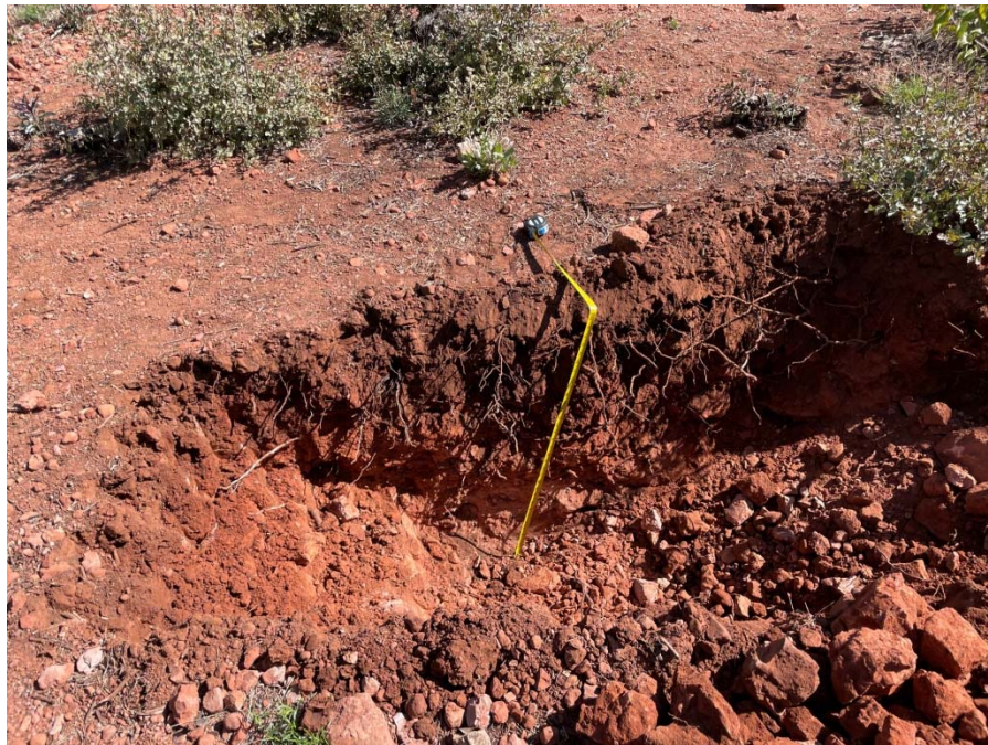
Photo 5 – Excavated Test Pit 3. Test Pit 3 was terminated at a depth of 2.5 feet due to backhoe refusal on hard mudstone bedrock. The soils encountered to a depth of 1.0 feet consist of red clayey silty gravel with cobbles, some sand, medium dense, damp, low PI. From 1.0 to 2.5 feet, the soils became lighter in color and dense, probable highly weathered mudstone bedrock.
