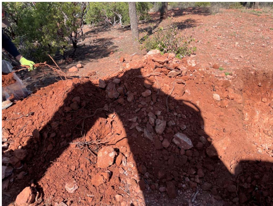
Photo 6 – View of material excavated from Test Pit 3 over the depth range of 0.0 to 2.5 feet, which appears to be primarily excavated mudstone bedrock.
