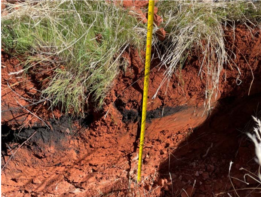
Photo 17 – Excavated Test Pit 9. Test Pit 9 was terminated at a depth of 2.5 feet due to backhoe refusal on hard mudstone bedrock – Supai Formation. . The upper 1.0 feet of red silty sandy gravel with cobbles is loose, moist, NP. A black layer of clayey sand with possible organics was encountered from 1.0 to 1.5 feet. Below 1.5 feet the soils became lighter in color, dense, and slightly damp, probable highly weathered mudstone bedrock.
