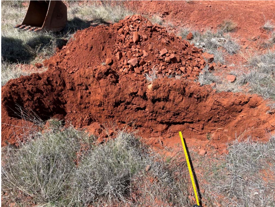
Photo 15 – Excavated Test Pit 8. Test Pit 8 was terminated at a depth of 2.5 feet due to backhoe refusal on hard mudstone bedrock. The soils encountered to a depth of 1.5 feet consist of red clayey silty gravel with cobbles, some sand, medium dense, damp, low PI. From 1.5 to 2.5 feet, the soils became lighter in color and dense, probable highly weathered mudstone bedrock.
