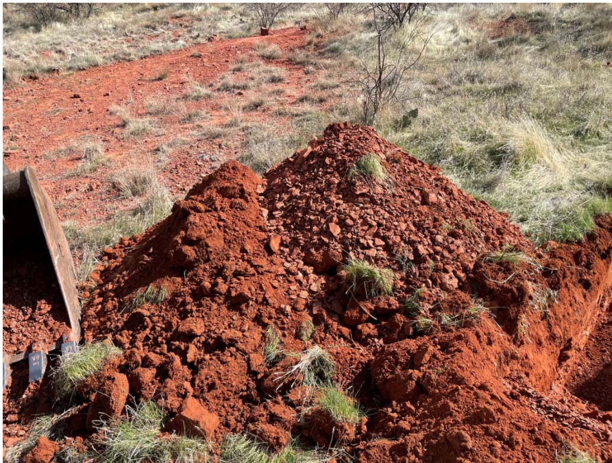
Photo 20 – View of material excavated from Test Pit 10 over the depth range of 0.0 to 2.0 feet.
