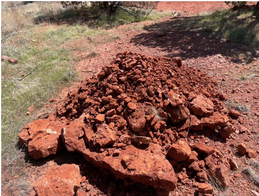
Photo 10 – View of material excavated from Test Pit 5 over the depth range of 0.0 to 1.0 feet, which appears to be primarily native soil and mudstone bedrock. Fragments of excavated mudstone bedrock can be seen in the
