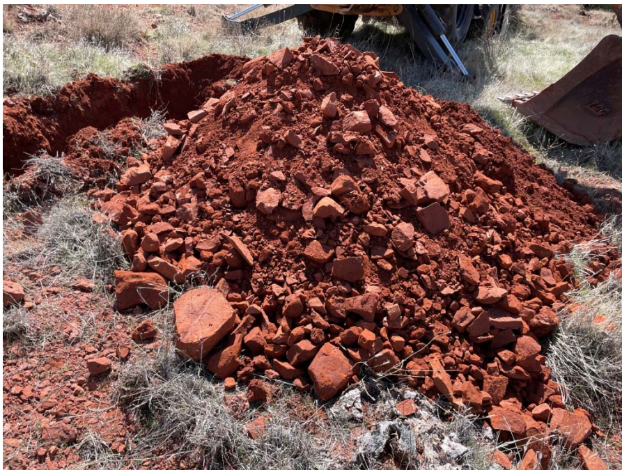
Photo 16 – View of material excavated from Test Pit 8 over the depth range of 0.0 to 2.5 feet, which appears to be primarily excavated native soils and mudstone bedrock.
