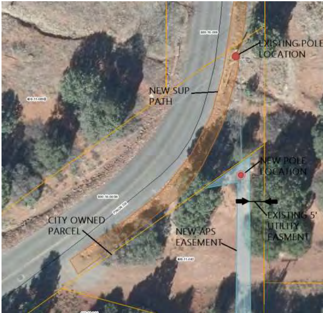
New and existing pole location
