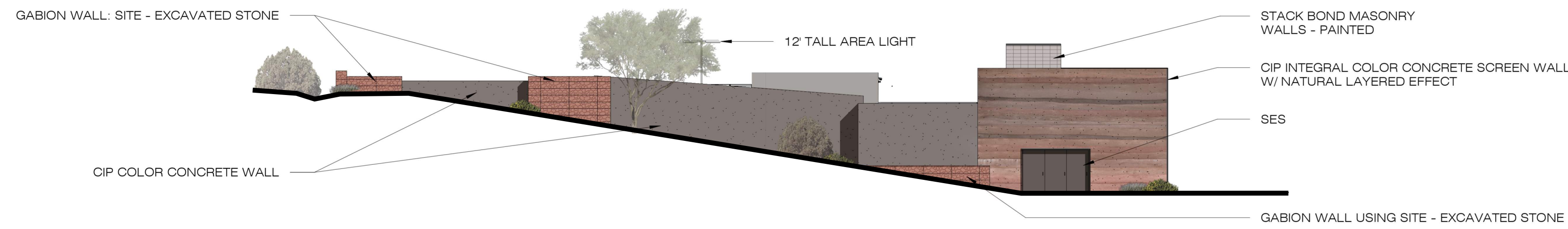
2 WEST - BUILDING ELEVATION 1/16" = 1'-0"
