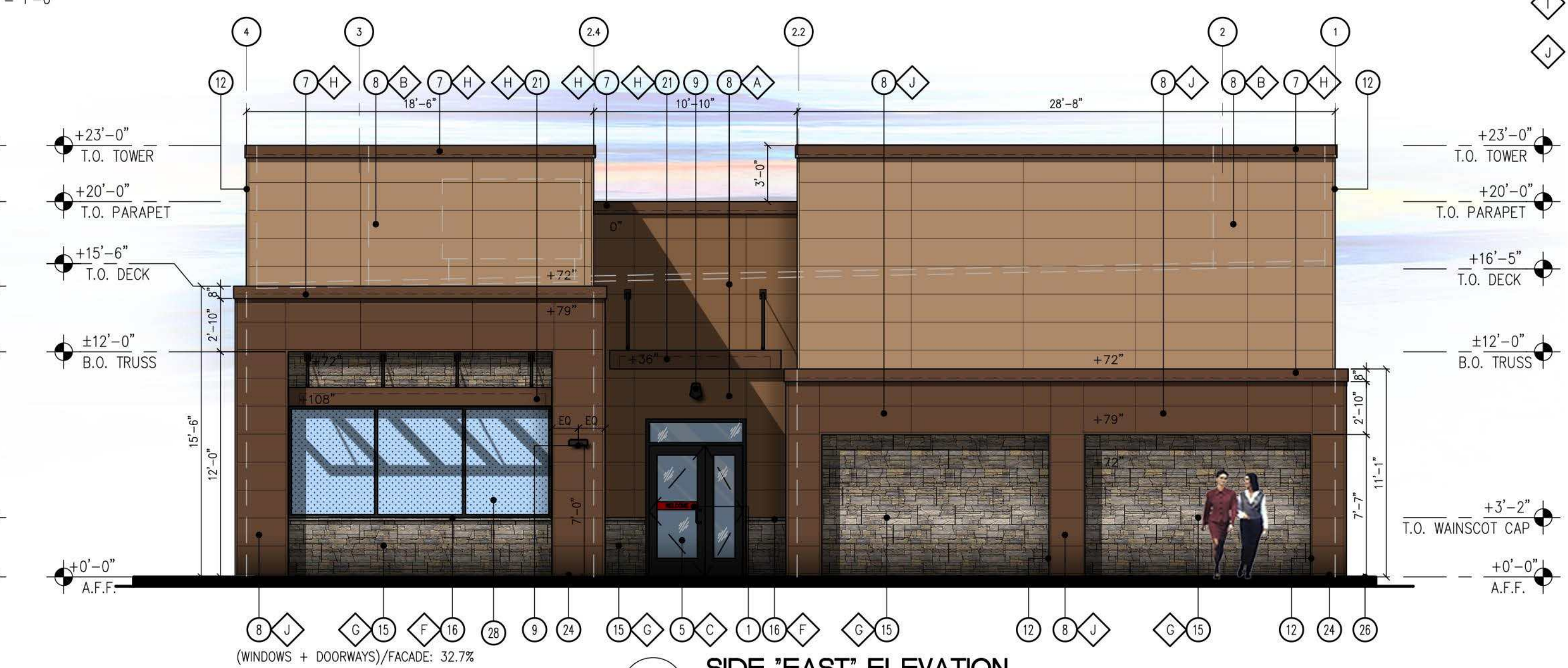
4 SIDE "EAST" ELEVATION
