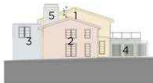
3.SPA - SOUTH ELEVATION SCALE: 1/16"=1'-0" Massing 2 area: 644.1sqft (41.4% of total area) Massing 3 area: 321.74 sqft (20.7% of total area) Total area: 1,556.4 sqft (100% of total area)
