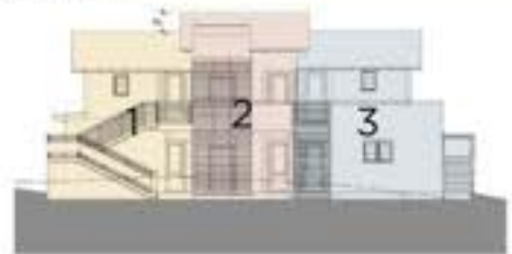
1. LODGING A - NORTH ELEVATION SCALE: 1/16"=1'-0" Massing 3 area: 517.8 sqft (34.9% of total area) Massing 2 area: 494.9 sqft (33.4% of total area) Total area: 1481.7 sqft (100% of total area)
