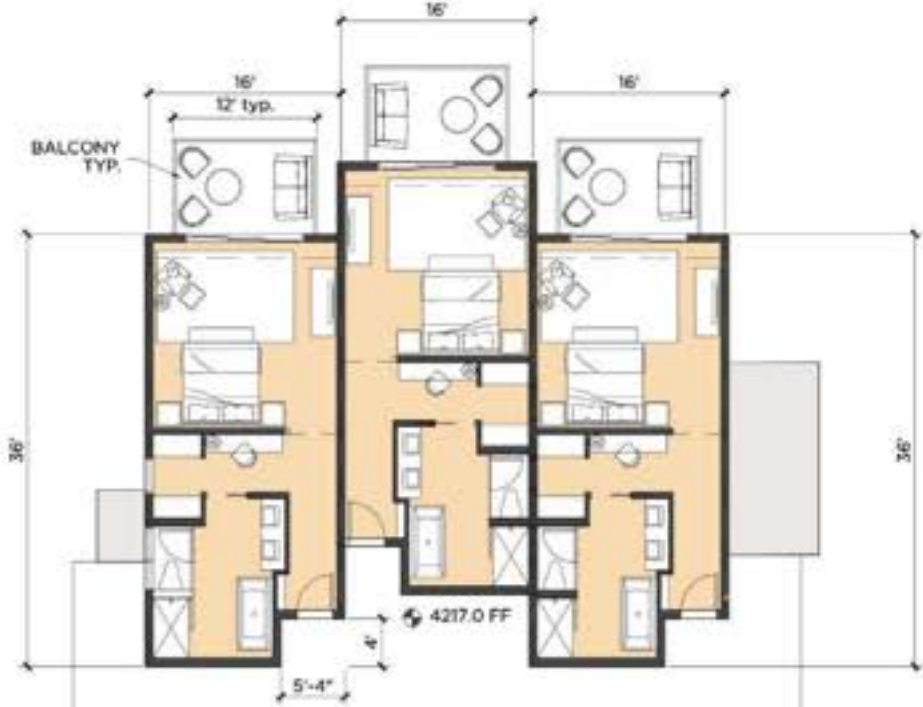
2. LODGING C - SECOND FLOOR PLAN SCALE: 1/8"=1'-0" GROSS AREA 1,699 SQFT FLOOD LINE FLOOD PLANE
