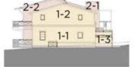
2. LODGING A - EAST ELEVATION SCALE: 1/16"=1'-0" Massing 1-1 area: 482.5 sqft (38.6% of total area) Massing 1-2 area: 365.1 sqft (29.2% of total area) Total area: 1,251 sqft (100% of total area)
