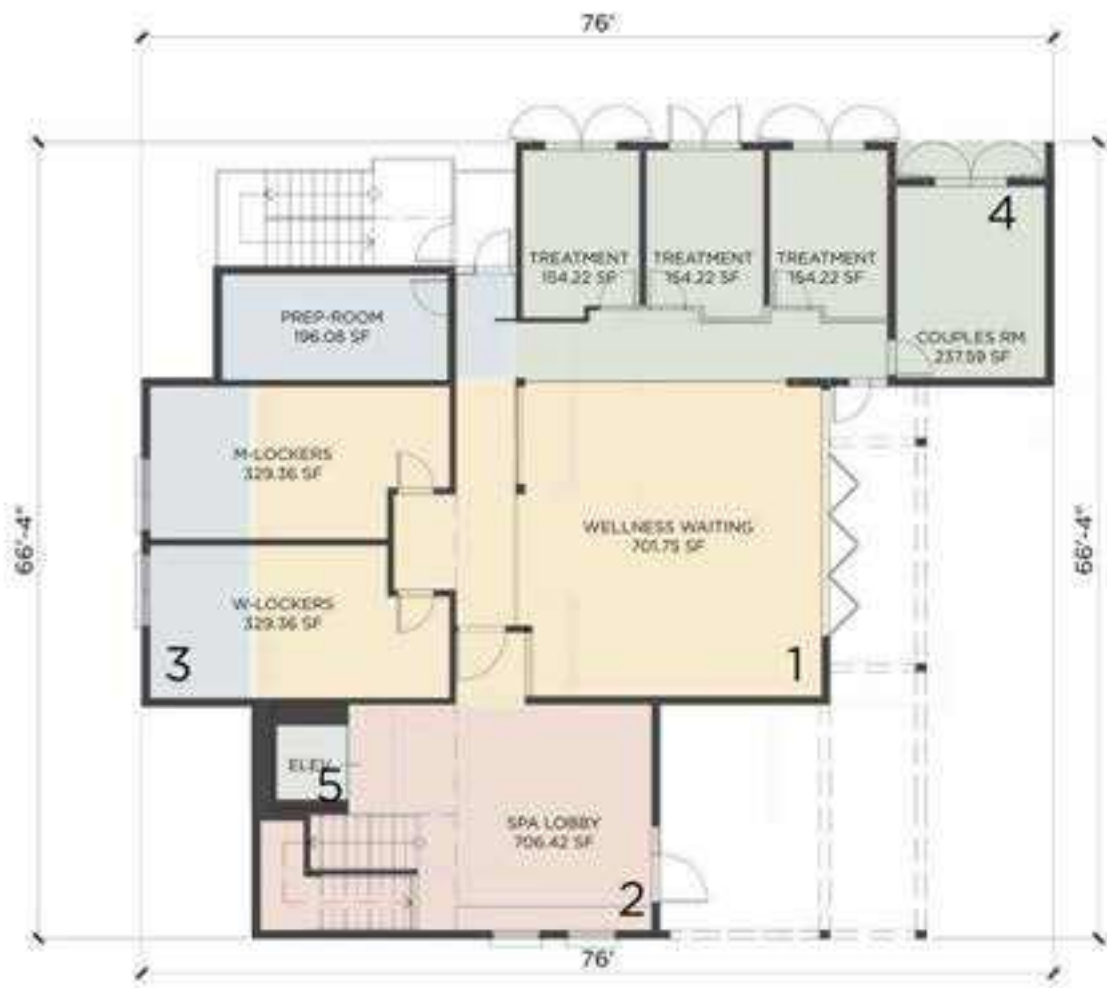
1.SPA - FIRST LEVEL FLOOR PLAN SCALE: 1/8"=1'-0" GROSS FLOOR AREA: 3,314 SQFT
