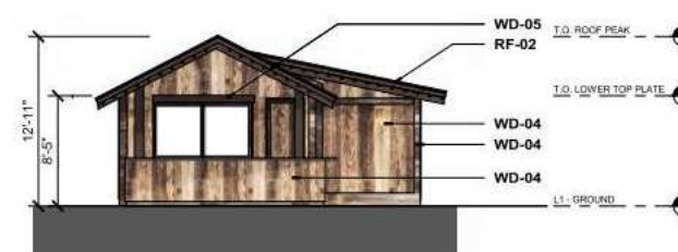
10. - SERVICE BUILDING - POOL NORTH ELEVATION 1/8" = 1'-0"
