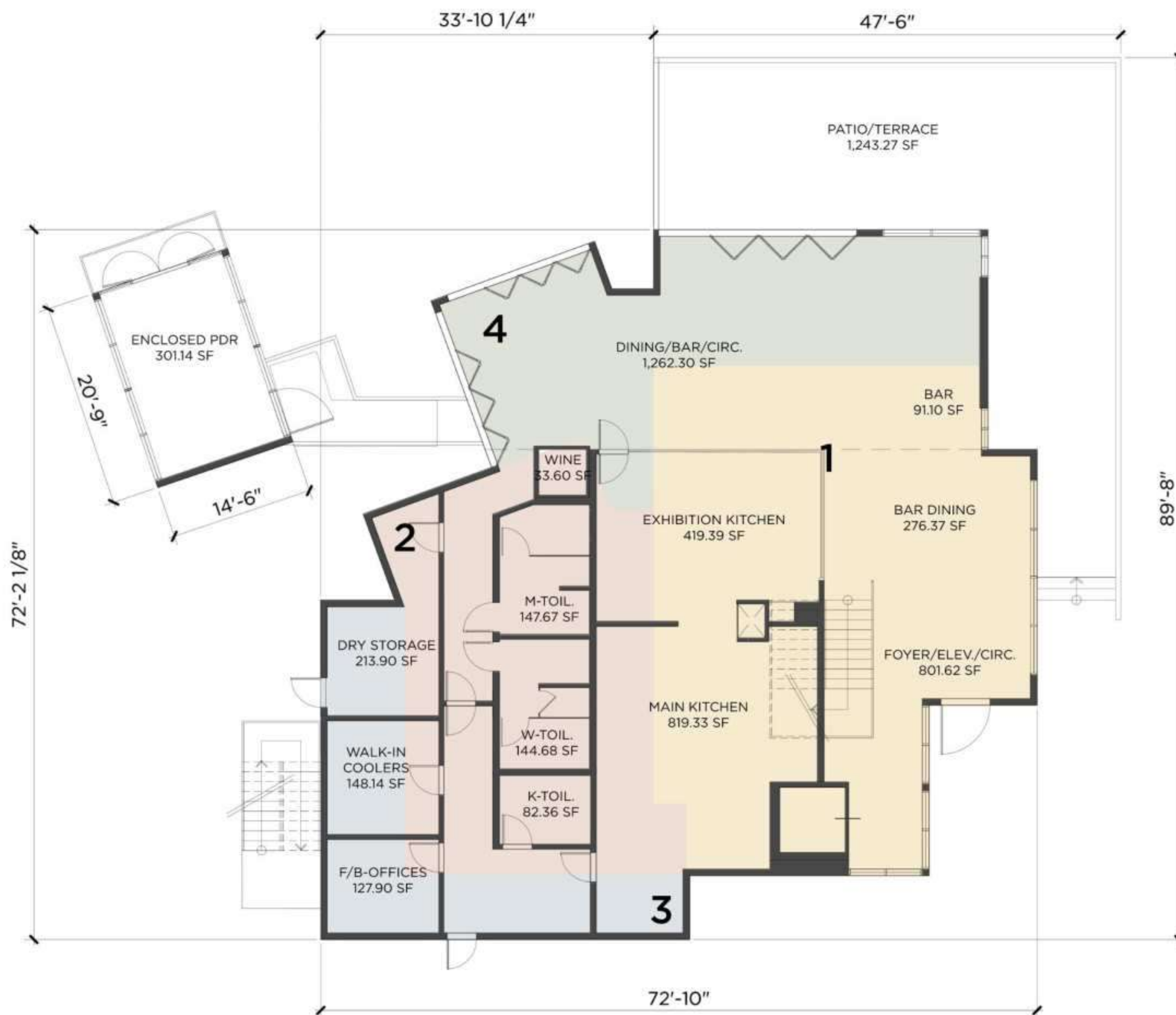
1. RESTAURANT - FIRST LEVEL FLOOR PLAN SCALE: 1/8"=1'-0" GROSS FLOOR AREA (EXCLUDES PDR): 4,198 SQFT
