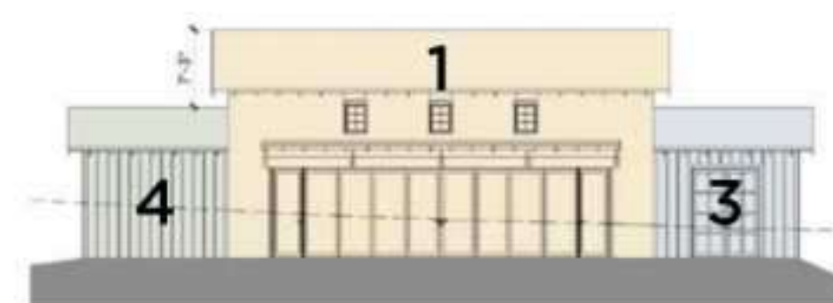
6. MEETINGROOM - NORTH ELEVATION SCALE: 1/16"=1'-0" Massing 1 area: 513.5 sqft (40.4% of total area) Massing 2 area: 361.3 sqft (28.4% of total area) Total area: 1271.9 sqft (100% of total area)
