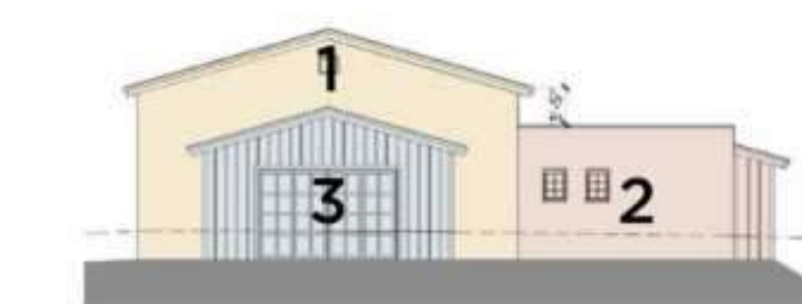
9. MEETINGROOM - WEST ELEVATION SCALE: 1/16"=1'-0" Massing 1 area: 292.1 sqft (30.3% of total area) Massing 2 area: 378.7 sqft (39.3% of total area) Total area: 964.6 sqft (100% of total area)
