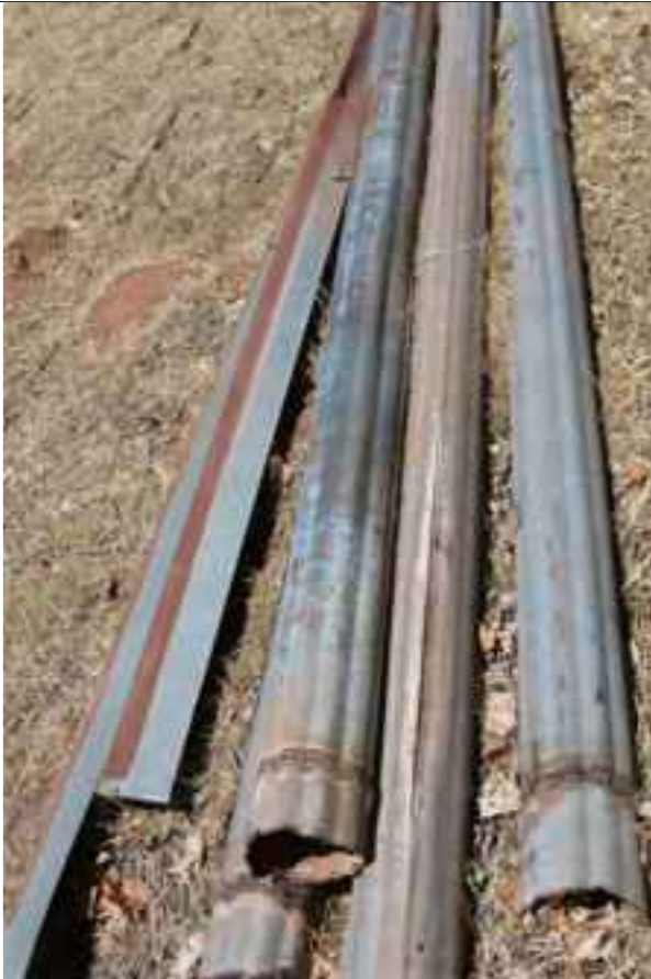
Corrugated Pipe Used for Farley/Steele Ditch (removed and stored at 115 Schnebly Hill Road)
