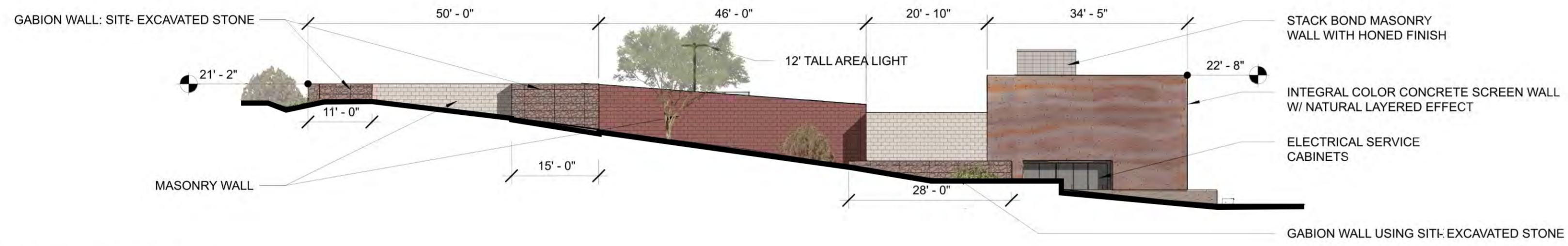
2 WEST -BUILDING ELEVATION 1/16" = 1'-0"
