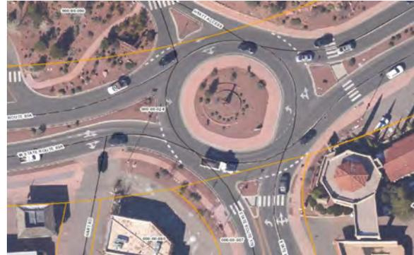
Metering also allows for safety benefits to pedestrians in crossings while controlling traffic at those peak hours of the day. The metered signals can be used to improve the flow of traffic on legs of the roundabout where long vehicle queues tend to form.
