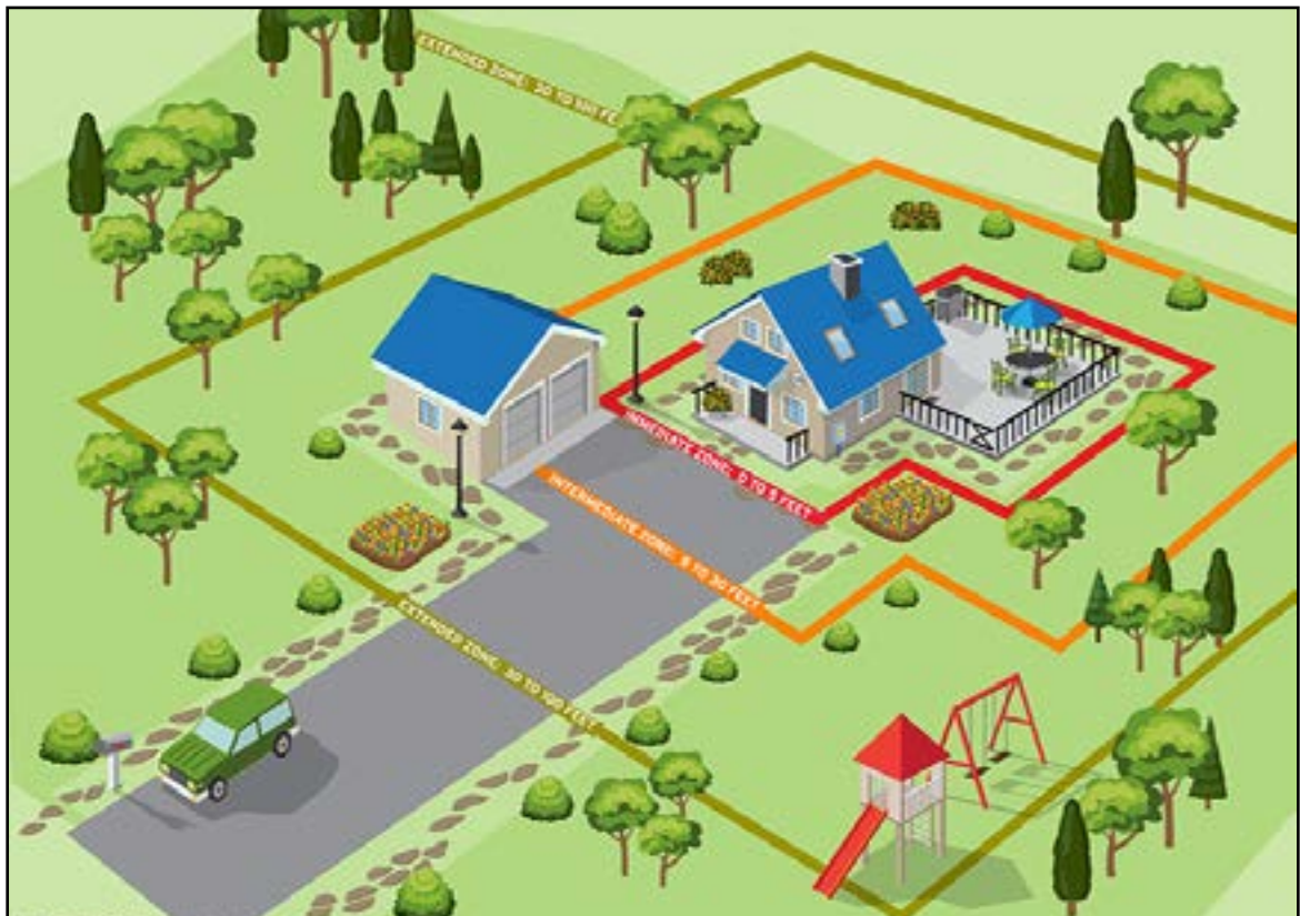
Figure 7.4. Clearance zones around homes and structures.
