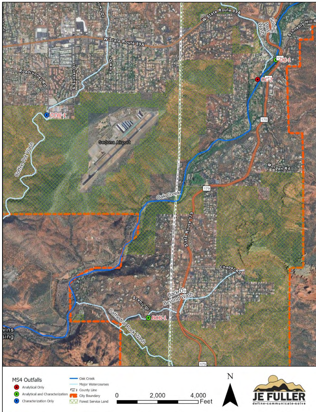
Figure 5-1: Identified Outfall Locations
