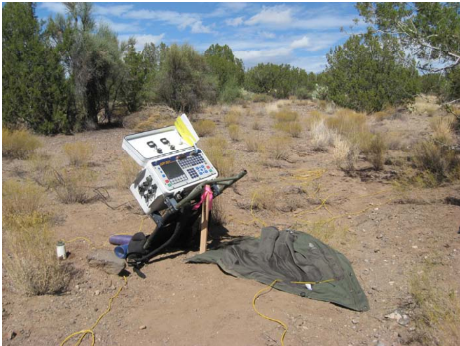
Photo 4. A good view of the portable receiver set up to record data a few hundred feet north of the potable water well. Note electrode in the ground.
